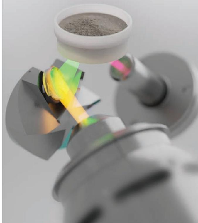
When the X-ray tube, secondary target, sample, and detector are aligned in 90° Cartesian Geometry, measurements have no background.
