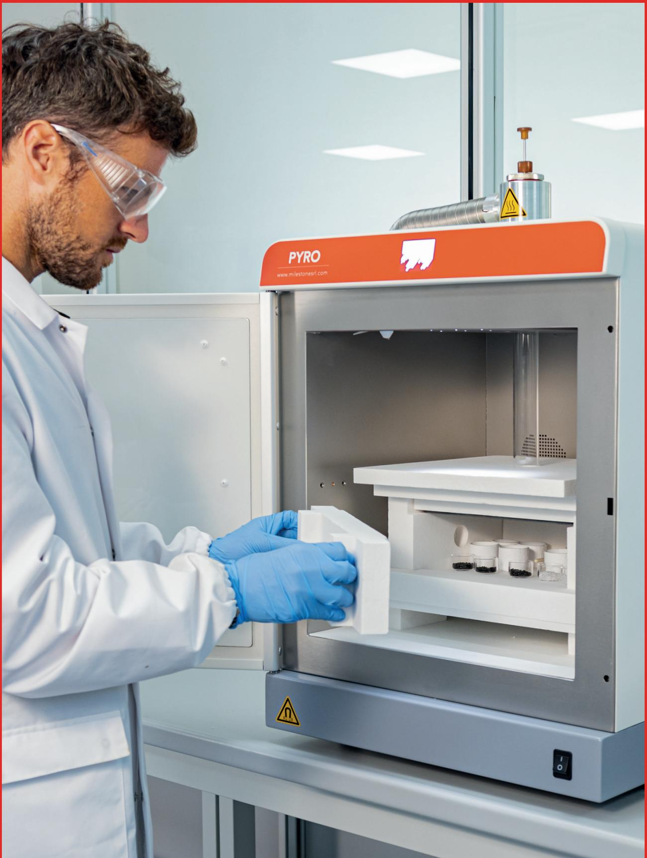
The PYRO is built to offer superior working conditions and a more efficient ashing procedure on a wide range of matrices. It incorporates in a single platform a rugged hardware, a reliable microwave-transparent muffle, an efficient exhaust, an accurate temperature control and a smart user interface.
