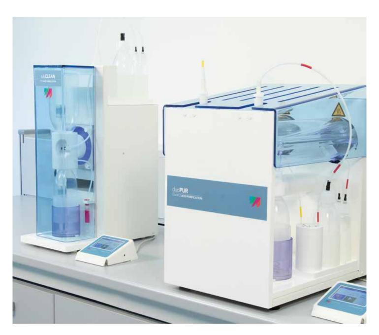
Milestone applied sub-boiling distillation technology in the duoPUR and SubCLEAN. The duoPUR has two quartz purification units and allows the purification of the most common acids such as HNO<sub>3</sub> and HCl, while the SubCLEAN has a single PTFE-TFM purification still, allowing the purification of HNO<sub>3</sub>, HCl and HF too.
